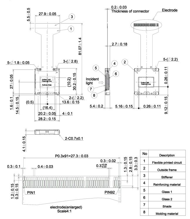
The rotaition angle of active area relative to H and V is ±1°
