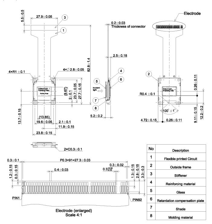
The rotaition angle of active area relative to H and V is ±1°
